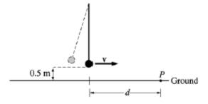
e) suppose the object undergoes this motion because it is the bob of a simple pendulum as shown above. If the object breaks loose from the string at the instant the pendulum reaches its lowest point and hits the ground at point P shown, what is the horizontal distance d that it travels?
