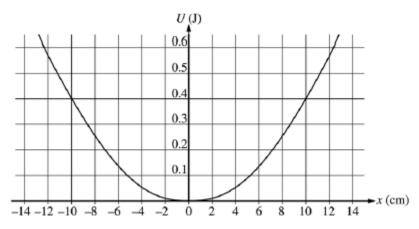
3) A 3.0 kg object subject to a restoring force F is undergoing simple harmonic motion with a small amplitude. The potential energy U of the object as a function of distance x from its equilibrium position is shown above. This particular object has a total energy E = 0.4 J.
