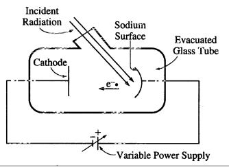
3) A sodium photoelectric surface with work function 2.3 eV is illuminated by electromagnetic radiation and emits electrons. The electrons travel toward a negatively charged cathode and complete the circuit shown above. The potential difference supplied by the power supply is increased, and when it reaches 4.5 V, no electrons reach the cathode.
