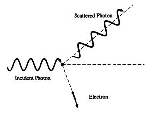
An x-ray photon of the maximum energy produced by this tube leaves the tube and collides elastically with an electron at rest. As a result, the electron recoils and the x-ray is scattered, as shown below. The frequency of the scattered x-ray photon is  $1.64 \times 10^{19}$  hertz.
